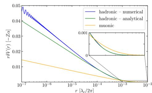
Figure 2. Comparison of muonic and hadronic Uehling potential for point-like nucleus [2].
